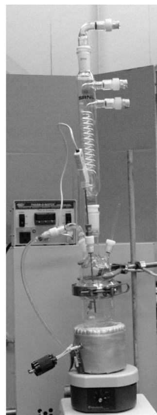
FIG. 2. Equipment for actual Tank A waste chemical cleaning test.
